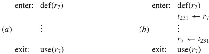
**FIGURE 11.7.** Moving a callee-save register to a fresh temporary.
